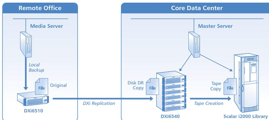
*Close integration with backup applications means reduced complexity for users. The DXi6500 works with NetBackup's OpenStorage API, for example to let users automatically manage data on disk and tape across sites using NetBackup policies. Data is moved by DXi systems—initiation, management, cataloging is through NetBackup.*
