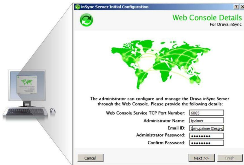
Overall, installation and configuration took about 20 minutes, including configuring the network ports so that users could access the inSync server from outside the Lab firewall, configuring storage on the server and creating user profiles with the Druva inSync web console, seen in Figure 4.
