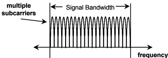
**Figure 5 OFDM Systems Transmit Data on Multiple “Subcarriers”**
