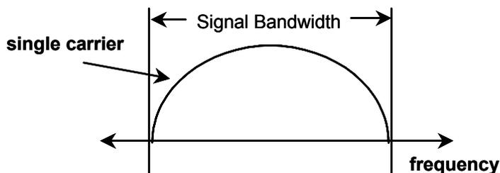
**Figure 3 CCK is a “Single-Carrier” Modulation Format**
