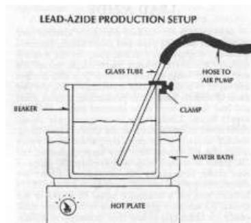
Solution A: Dissolve 2 grams of sodium azide and 60 milligrams of sodium hydroxide (lye) in 70 milliliters of distilled water.
