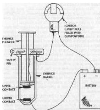
plunger is threaded through it. The syringe is assembled, and the plunger is pushed down until the contacts are about 1/8 inch apart. A hole is drilled horizontally through the plunger at this point for the safety pin. The excess wire is pulled through the hole in the finger rim, and this hole is sealed with glue. There must be enough slack in the wire so that the
