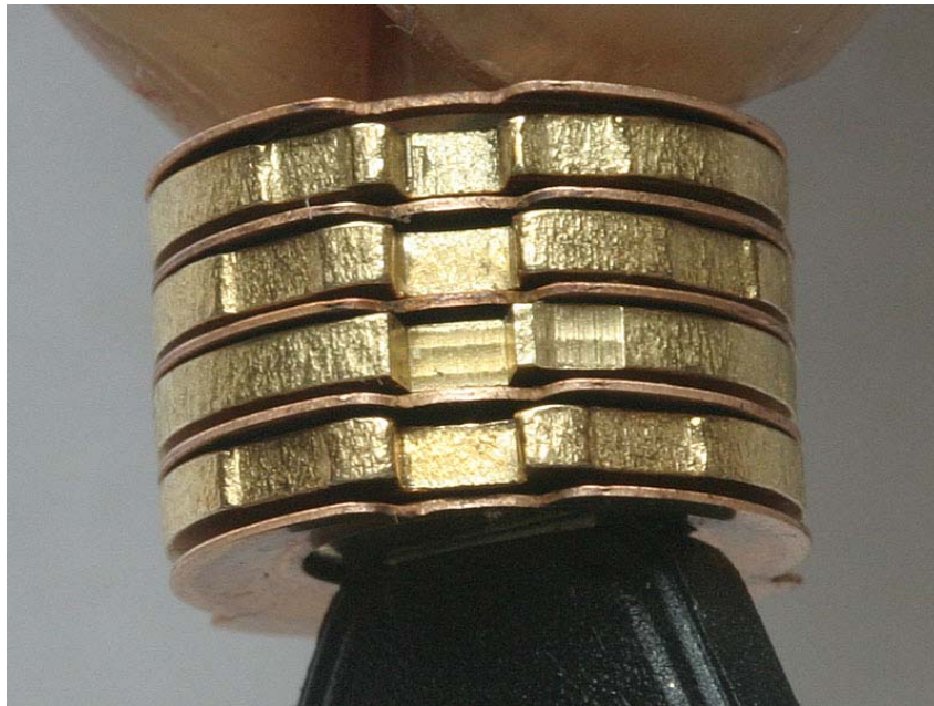
View on the false gates / notches in Classic disc number 3
