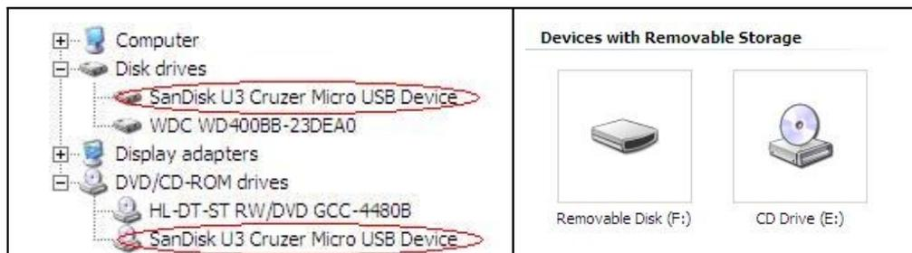
Figure 1: The two devices under device manager and as Removable Disk (F:) and CD Drive (E:)
