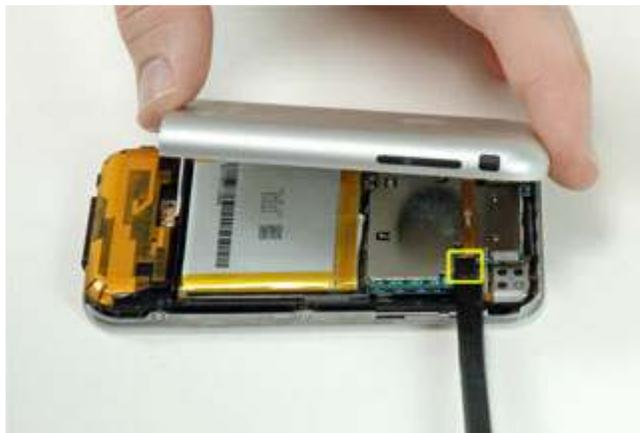
After you removed this you will notice a metal shield over the baseband chips. This needs to be removed as well. Use a tiny screwdriver or something similar to carefully lift it of.
