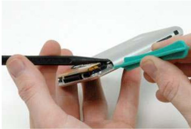
Slide the iPod opening tool along the edge of the case, releasing the three tabs. The rear panel is still attached to the iPhone by the headphone jack cable, so don't entirely remove the rear panel from the iPhone just yet.
