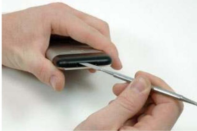
Insert an iPod opening tool in the gap between the antenna cover and the front bezel. The wedge should be pointing towards the antenna cover. Slide the tool around the corner and up until you reach the metal backing. Repeat the same procedure on the other side of the dock connector.
