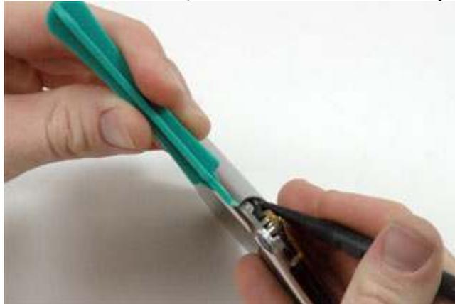
Repeat the same procedure on the other side of the iPhone to insert the iPod opening tool into the case. On this side, there are only three tabs to free, as there is no tab near the buttons.
