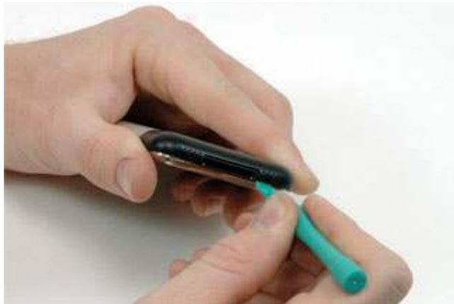
Grasp the antenna cover on either side and slide it up and away from the iPhone. This requires some force. If it does not come free, ensure that the antenna cover is lifted up enough to free the catches.
