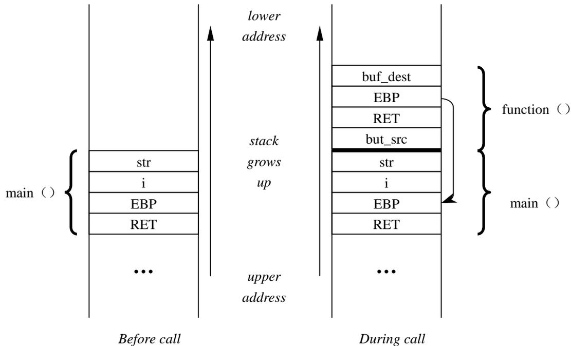
We can see from this figure that the content of array *str* (256-character 'a's, i.e., 0x616161...) has already overwritten all the former contents from *buf\_dest* to *buf\_dest*+256, including the EBP and RET saved when function calling. So when the function exits, it will return to 0x61616161, the segment fault occurred.
