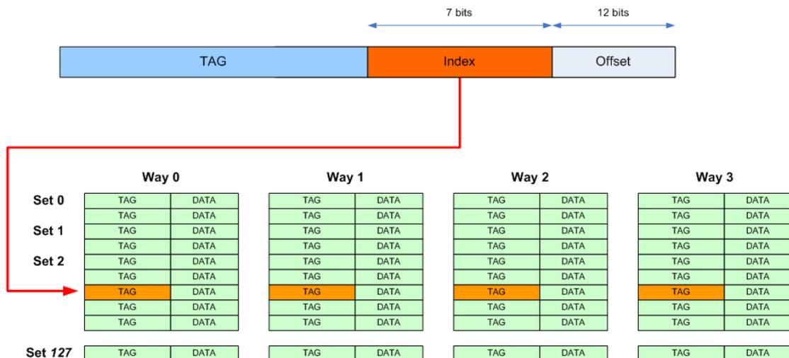
Figure 4.1: Illustration of the L2 TLB organization [Rut07b]
