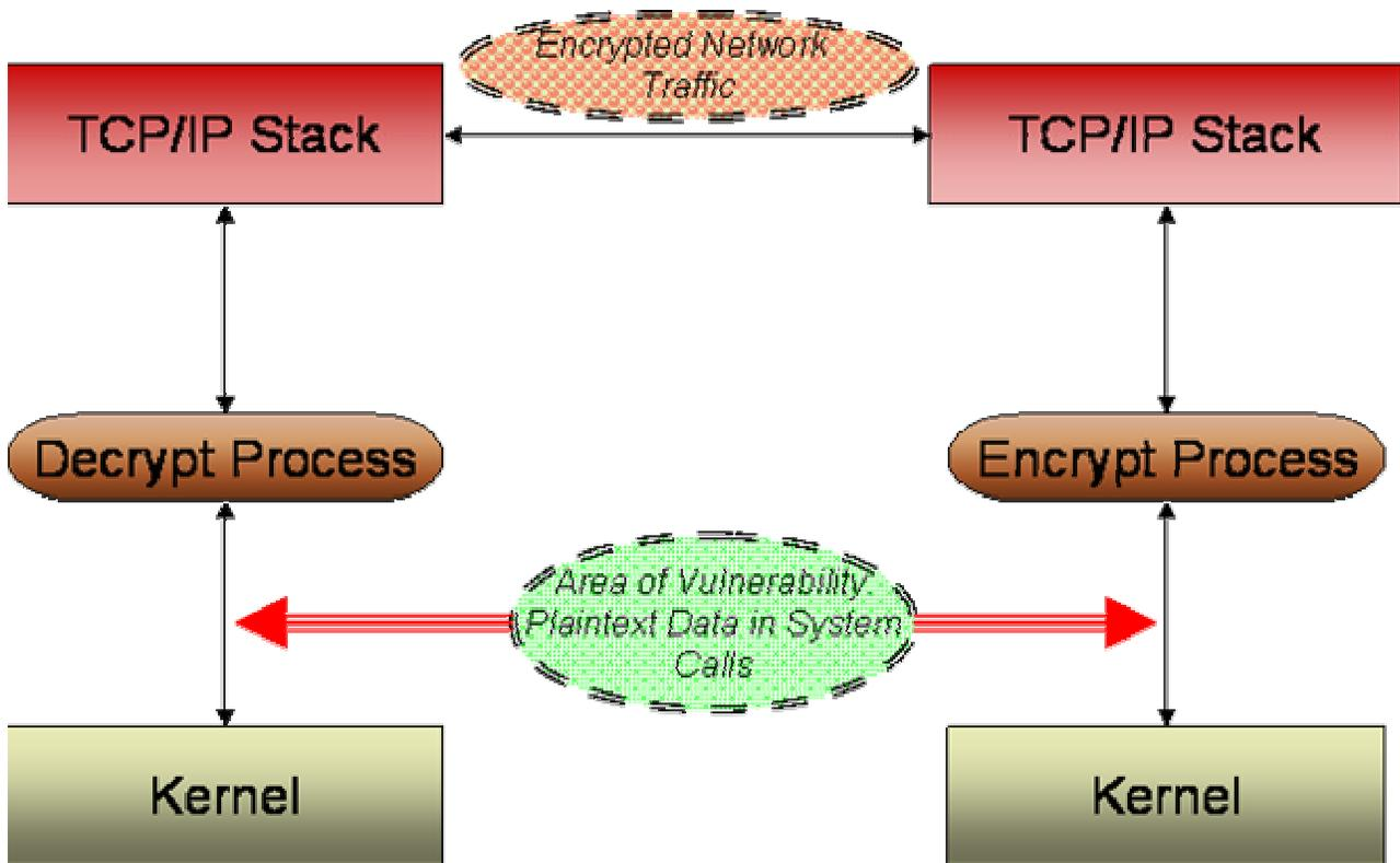
Figure 2. The encrypted communication process. Data sent over the wire is unreadable, but if someone can tap into the system calls, they can see the data in plaintext before or after encryption has taken place.
