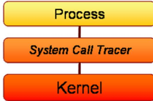
Figure 1. This diagram is an illustration of the virtual location of the system call tracer. It sits between the kernel and the process so it can see the data passed between them.
