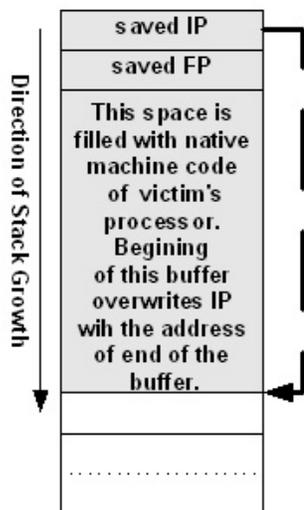
Figure 5: Typical Buffer Overflow in Action
